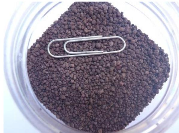
**Iron chloride/iron oxide pellets
