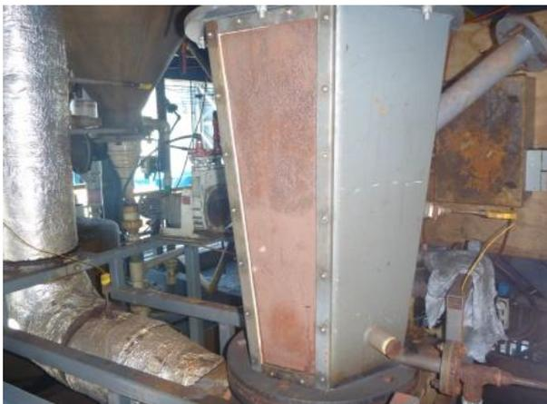
**The fluid bed evaporator producing iron oxide/iron chloride pellets from pickle liquor and furnace dust**
