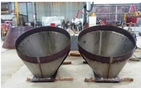
Fabrication of product silos.
