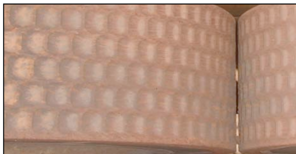
The briquetter rolls are 630 mm in diameter and weigh 3 tonnes each.
