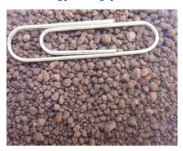
Detail of iron chloride/iron oxide pellets (1-4mm in diameter)
