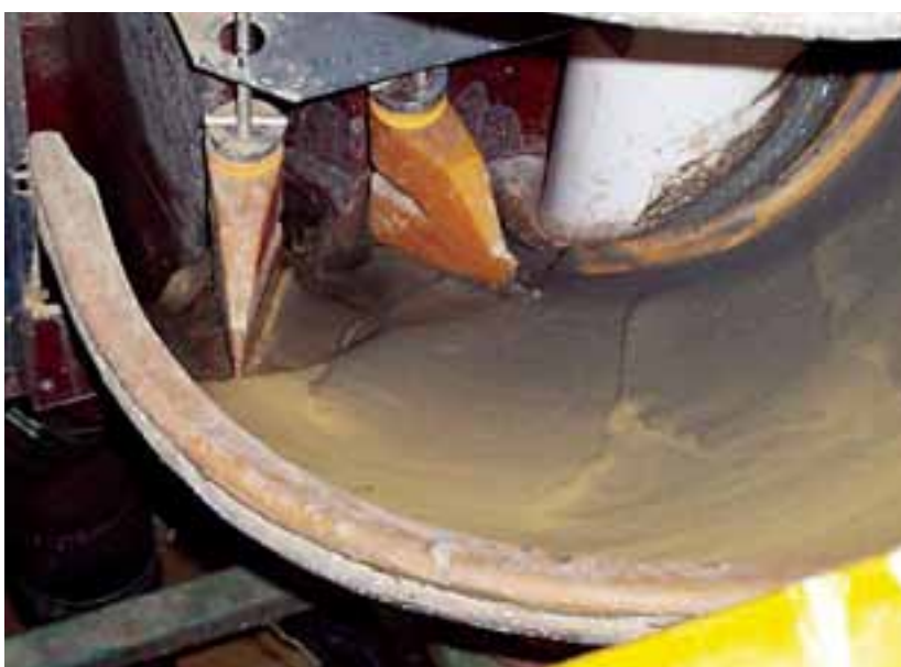
↑ Spiral separation of WIM 150 heavy minerals
