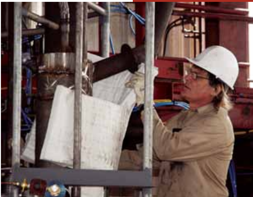
↑ Fine mineral agglomerates ↓ Jon Trigger insulating the metalliser
