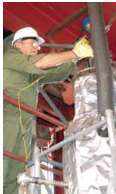
↑ John Cox adjusts thermocouples on the metalliser
