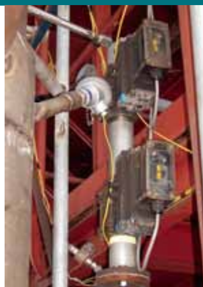
↑ Double dump valve ↓ John Winter operating metalliser
