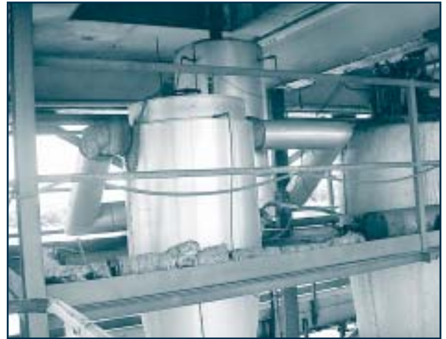
Off-gas from the LTR roaster (front) passes through the afterburner (rear) which ensures environmentally acceptable emissions.
