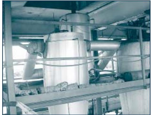
Off-gas from the LTR roaster (front) passes through the afterburner (rear) which ensures environmentally acceptable emissions.
