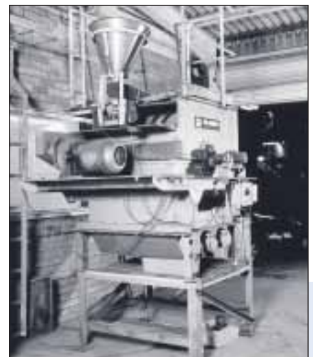
Multi-pole agitated drum magnet at the pilot plant
